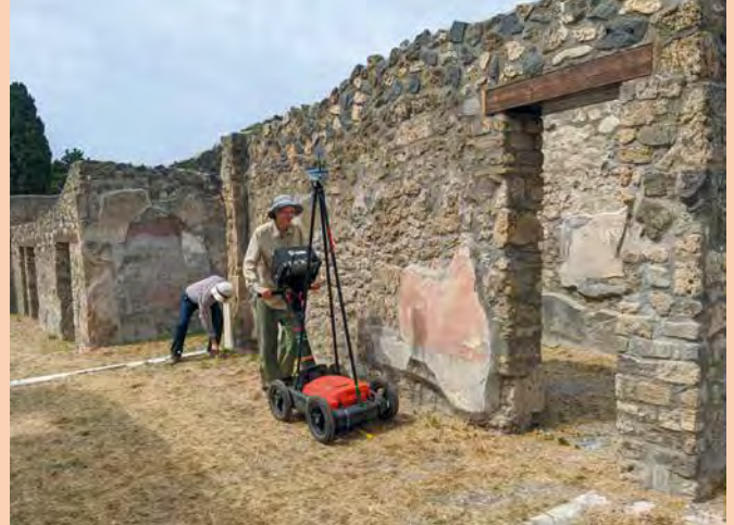
Ground-penetrating radar (GPR) investigations at the Insula del Citarista (I 4), one of the central city blocks of Pompeii, Italy.
